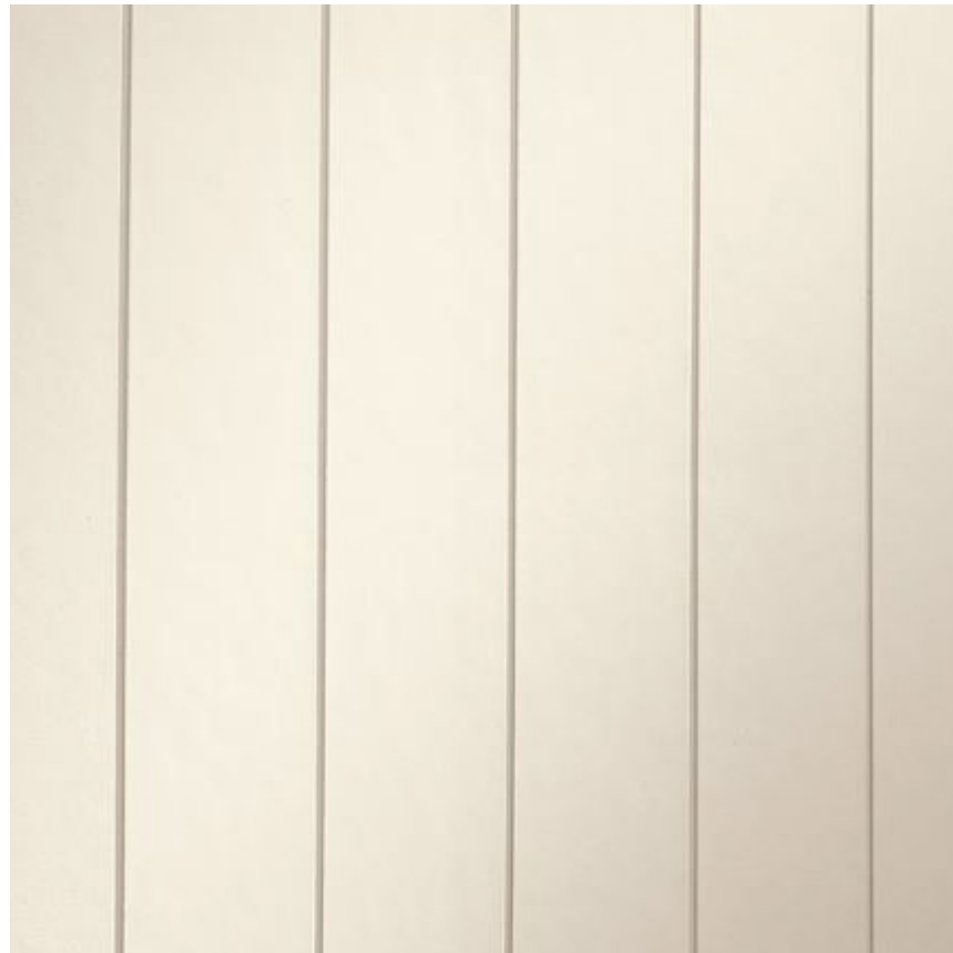
SIDING: 8" REVERSE BOARD & BATTEN CEMENTITIOUS SIDING WITH 1/2" REVEAL; SMOOTH FINISH, NO WOOD GRAIN; PAINTED SHERWIN WILLIAMS ALABASTER
